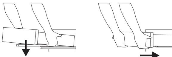
Insertion: support the rails and push until the end.
